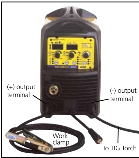
Fig 9 Cable and hose connections for TIG welding
